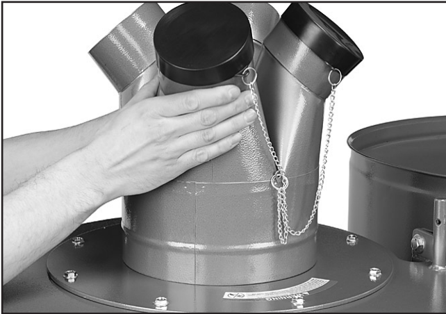
Figure 8. Installing 4-in-1 inlet adapter.
